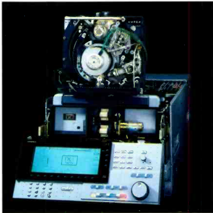
The tape drive is built with a modular architecture and remains operational even with maintenance access to the circuitry.
